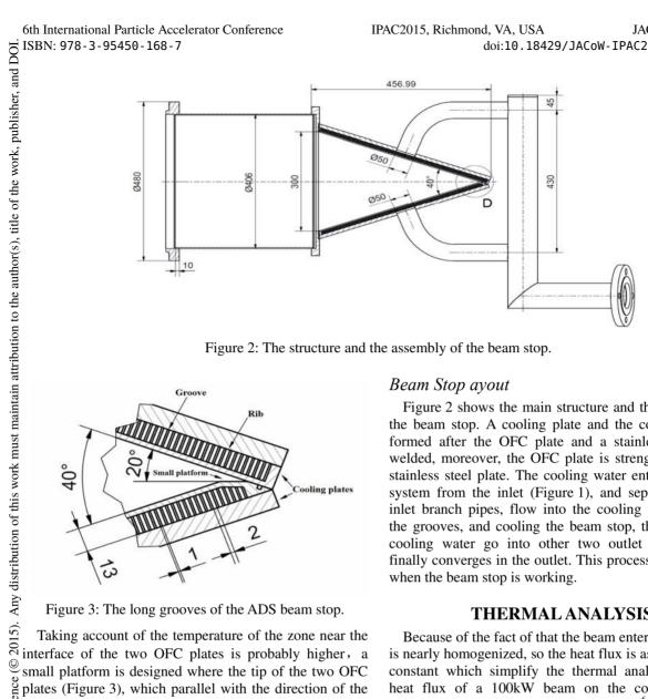
Figure 2: The structure and the assembly of the beam stop.
