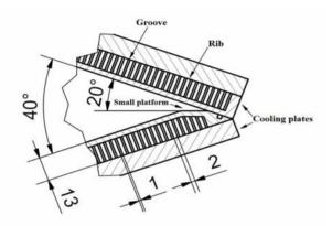
$\bigcirc$  interface of the two OFC plates is probably higher, a  $\bigcirc$  small platform is designed where the tip of the two OFC plates (Figure 3), which parallel with the direction of the  $\bigcirc$  beam. Consequently, several grooves is increased in the  $\underset{\mathfrak{S}}{\circ}$  tip, and more heat can be taken away avoiding the high temperature of the tip and even the destroy of the copper  $\mathcal{H}_{\text{relation}}$ plates.
