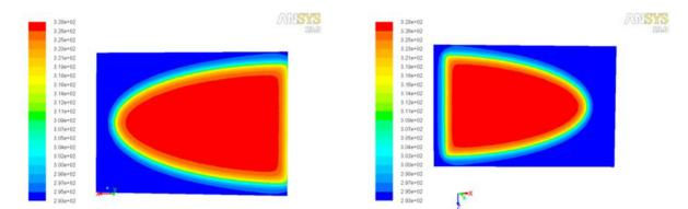
Figure 5: The contours of beam hit surface of the upper cooling plates and lower cooling plates.
