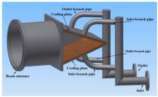
Figure 1: The structure of the ADS beam stop.
