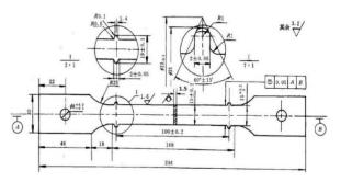
Figure 4: Sample dimensions for creep experiment.
