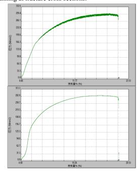
Figure 2: Tensile curve (U: at 25 °C; D: at 100 °C).
