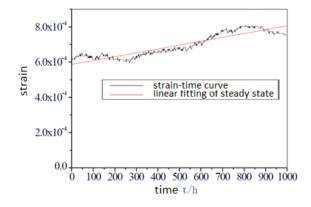
Figure 6: Linear fitting for creep curve at 100  $^{\circ}\mathrm{C}$  and 60 MPa.
