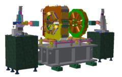
Figure 4: Vibrating wire alignment system model.
