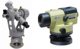
Figure 4: The Theodolite and Level.
