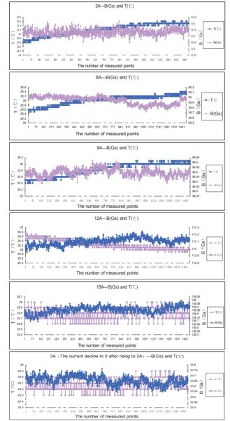
Figure 6: The magnetic field and temperature values under different current.
