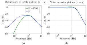
Figure 4: Closed-loop system response comparison of PI control and "PI+DOB" control. From left to right: (a) Disturbance to cavity pick-up  $(d \rightarrow v)$ ; (b) Noise to cavity pick-up  $(n \rightarrow y)$ .
