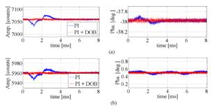
Figure 6: Measured RF field for the amplitude (left) and the phase (right) in the cavities of the injector in the presence of  $800\text{-}\mu\text{A}$  beam loading. Red and blue waveforms in each subplot represent the PI control and the PI+DOB control, respectively. From top to bottom: (a) Inj. 1, (b) Inj. 2&3.
