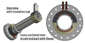
Figure 1: Design of dipole type CCIPM for the fabrication.
