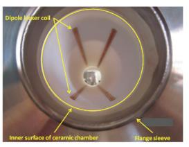
Figure 4: The inner surface view of the complicated CCIPM.
