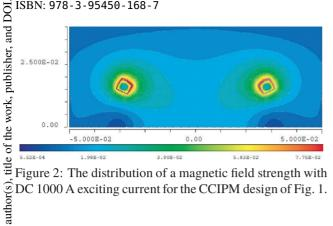
Figure 2: The distribution of a magnetic field strength with DC 1000 A exciting current for the CCIPM design of Fig. 1.
