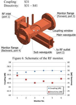
Figure 7: Coupling and directivity of RF monitors in the prototype module
