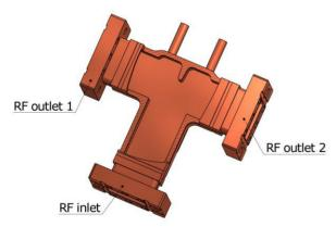
Figure 8: Schematic of the H-plane splitter.
