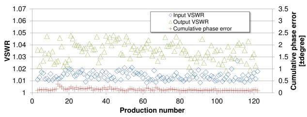
Figure 2: Input / Output VSWR and cumulative phase error of 120 S-band structure for PAL-XFEL after tuning. #nobuyuki shigeoka@mhi.co.jp
