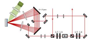
Figure 4: Thin-disk multi-pass amplifier with cavity.
