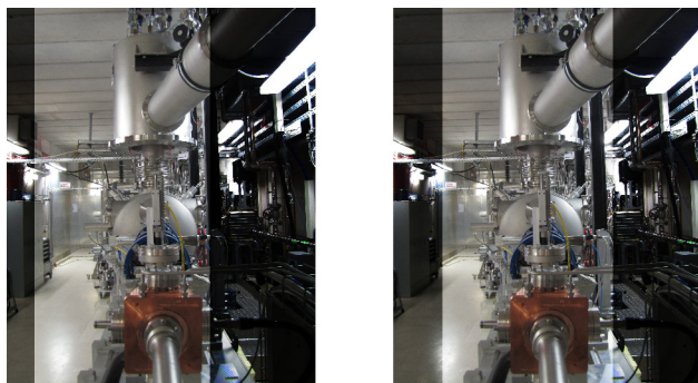
Figure 4: Composite photographs with front view of the ELBE cryomodules. The shaded areas refer to the respective position of each of the two cryomodules foreseen for MESA.
