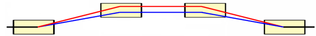
Figure 1: Schematic of a D-type bunch compressor. Particles with higher energy (blue) receive a smaller deflection in the dipole magnets (i.e. travel along a shorter path) than particles with a lower energy (red). For the correct initial energy distribution along the bunch, a bunch length compression can be achieved.
