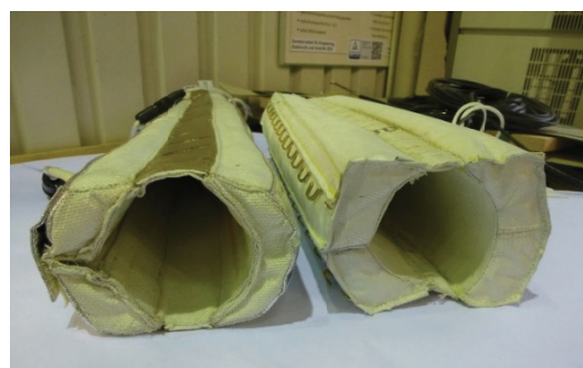
Figure 6: Special design of the dipole heater jackets.
