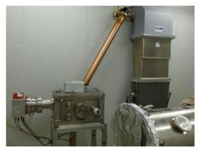
Figure 3: 325 MHz test cavity structure on support.
