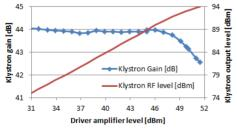
Figure 10: Driver level and klystron output power level.
