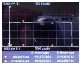
Figure 4: Undisturbed 0.4 ms long 45 kW RF pulse.
