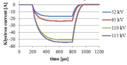
Figure 9: Klystron current measured in the oil tank.
