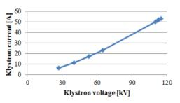
Figure 8: Klystron current vs. klystron voltage.
