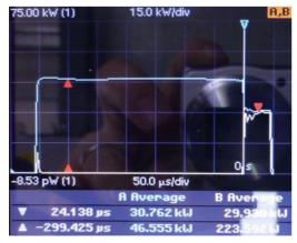
Figure 6: No amplifier shutdown with 21 cm extension.
