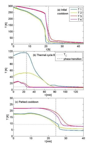
Figure 2: Temperatures measured during initial cooldown Figure 2: Temperatures measured during limital cooldown  $\xi$  (a), a thermal cycle (b) and parked cooldown (c). The dotted line indicates T<sub>c</sub> (9.2 K). The dashed line indicates the time when the first sensor dropped below T<sub>c</sub>.
