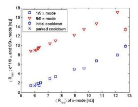
Figure 4:  $R_{res}$  obtained for the  $8/9\pi$  and  $1/9\pi$  mode as a function of  $R_{res}$  obtained for the  $\pi$  mode. Linear regression leaving out the initial cooldown results in:  $R_{8/9\pi} = 1.2 \cdot R_{\pi} + 1.8 \text{ n}\Omega$  and  $R_{1/9\pi} = 1.0 \cdot R_{\pi} - 4.7 \text{ n}\Omega$ .
