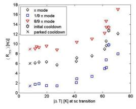
Figure 3: R<sub>res</sub> measured with the three passband modes as a function of  $\Delta T$  along the cavity at the onset of sc phase transition. The lowest R<sub>res</sub> was achieved in the center cells following the cycle 1 and the parked cooldown (1.4 n $\Omega \triangleq$  $Q_0 > 10^{11}$  at 1.5 K).
