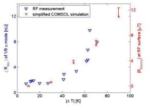
Figure 5: Magnetic field at the RF surface simulated for different temperature differences in combination with the RF data of Figure 3. The red bars indicate the magnetic field that is obtained assuming a 30% higher thermopower, corresponding roughly to the uncertainty in our measurement of the Nb thermopower [3].
