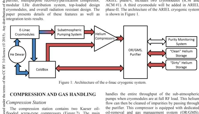
Figure 1: Architecture of the e-linac cryogenic system.
