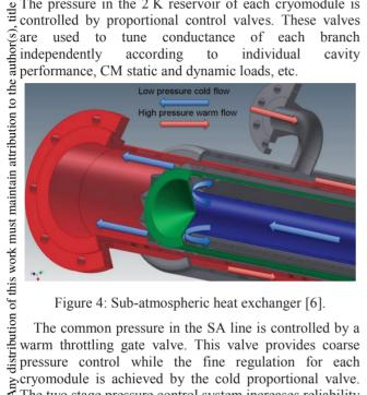
Cryomodule is achieved by the cold proportional valve. The two stage pressure control system increases reliability  $\dot{\mathfrak{S}}$  and flexibility of the operation.
