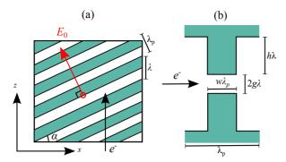
Figure 1: Dielectric grating structure. (a) Grating structure viewed from above. The electron beam travels in z, and the laser wavefront vector is incident in the -y direction. (b) Grating profile, highlighting dimensions varied in these simulations.
