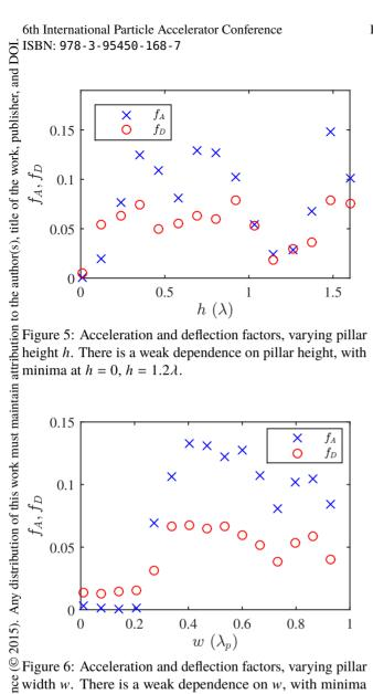
Figure 6: Acceleration and deflection factors, varying pillar
