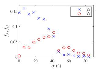
Figure 4: Acceleration and deflection factors, varying rotation angle  $\alpha$ . As  $\alpha \to 0$ , the geometry approaches the grating accelerator without significant deflection.
