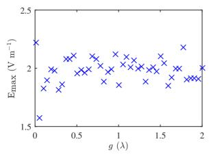
Figure 2: Maximum electric field in the structure, varying gap. For the dielectric grating structures analysed here, the maximum electric field  $E_{\rm max}$  is found at the surface between the vacuum and the dielectric. The value of  $E_{\rm max}$  rises sharply as g increases from zero, towards a constant value.
