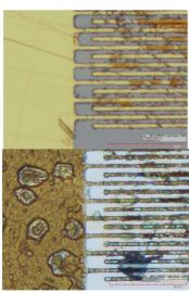
Figure 3: IDT device on GaAs substrate before (upper E rigure 5: ID1 device on GaAs substrate before (upper picture) and after (lower picture) heat processing at about \$550C [10].
