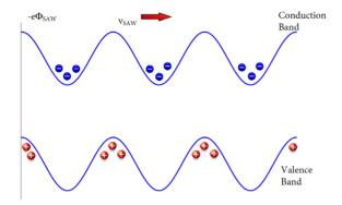
Figure 2: Band distortion, dynamical formation of type-II band structure in GaAs and charge carrier separation under piezoelectric potential  $\Phi_{SAW}$  of propagating SAW.
