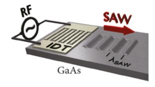
Figure 1: Generation of SAW on a piezoelectric substrate with an interdigital transducer (IDT) powered by an RFsource.
