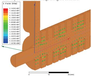
Figure 2: Shows the input coupler and the first 9 cells of the un-damped crab cavity prototype. The electric field is plotted for an input power of 13.35 MW.
