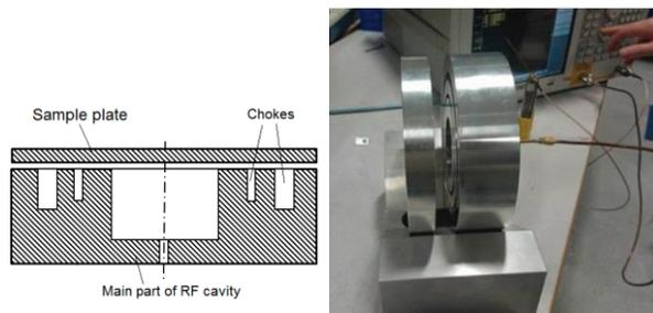
Figure 3: The 3.9 GHz aluminium prototype cavity.
