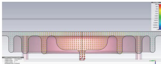
Figure 1: Electric field map of the three-choke cavity.
