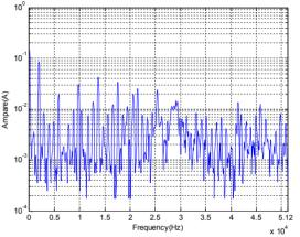
Figure 2: Current ripple in dc mode (frequency from 0 to 51.2 kHz).
