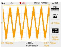
Figure 4: Using the negative output line and ground line of the AC source connection to measure the current.
