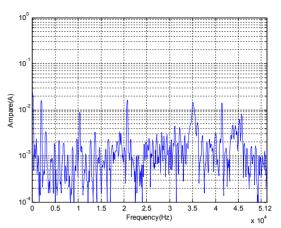
Figure 8: Current ripple in the dc mode with an added common-mode filter (frequency from 0 to 51.2 kHz).
