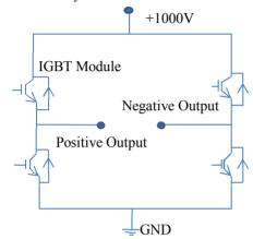
Figure 3: Topology of the dipole power supply.
