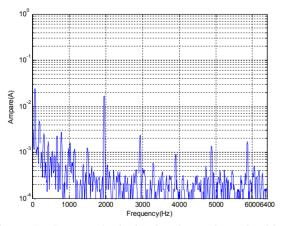
Figure 7: Current ripple in the dc mode and with an added common-mode filter (frequency from 0 to 6.4 kHz).
