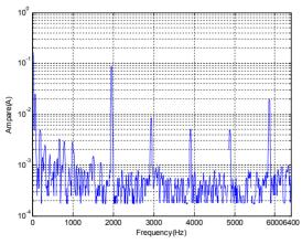
Figure 1: Current ripple in the dc mode (frequency from 0 to 6.4 kHz).
