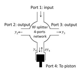
Figure 1: The 4 port network proposal for RF splitter.
