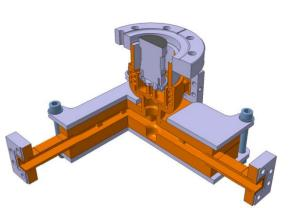
Figure 6: Mechanical design of the variable RF splitter.
