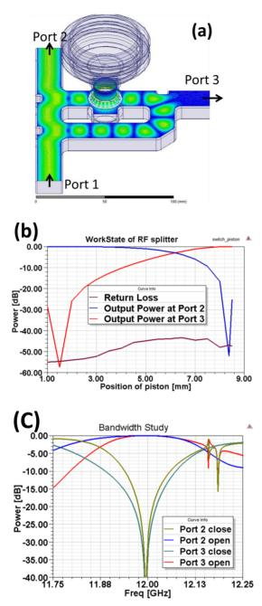
Figure 5: RF splitter design using 20 mm x 12 mm waveguide: (a) geometry; (b) power obtained at each port versus position of piston; (c) bandwidth plots.
