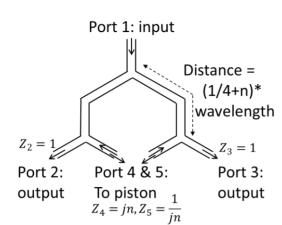
Figure 2: The 5 port network proposal for RF splitter.
