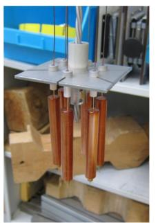
Figure 4: Centring plate and weights for the anodes
