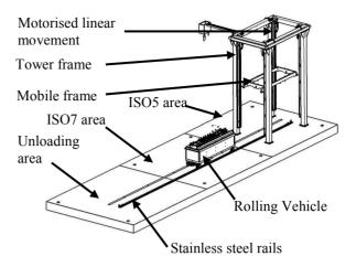
Figure 3: The specific assembly tooling.
