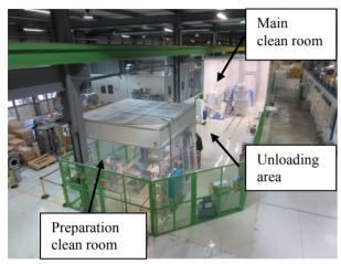
Figure 2: The HIE-Isolde cryo-module assembly facility.
