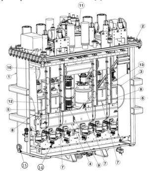
Figure 1: The complete HIE-ISOLDE high-β cryomodule; 1 Vacuum vessel lower box, 2 Vacuum vessel top plate assembly, 3 Thermal shield lower box, 4 Support frame, 5 Suspension end plate, 6 Tie-rod, 7 Inboard cavity, 8 Outboard cavity, 9 Down tube to solenoid, 10 Helium vessel, 11 Chimney assembly, 12 Support frame cooling supply, 13 Support frame cooling return, 14 Mathilde targets, 15 Mathilde viewport.
