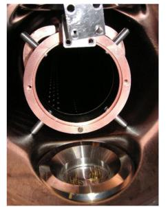
Figure 1: Picture of the a-C coated beam screen during reinstallation on February 2014.
