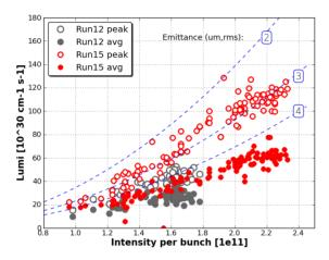
Figure 2: Peak and average luminosity for all stores as a function of bunch intensity. Peak luminosity in Run 12 saturated at  $50 \times 10^{30} cm^{-1} s^{-1}$  due to beam-beam induced emittance blowup. Electron lens compensation and improved off-momentum DA allowed higher luminosity in Run 15. The blue dashed lines are curves of constant emittance.
