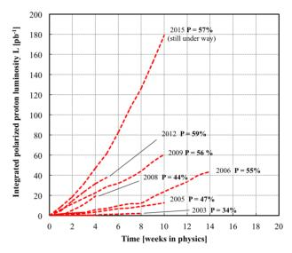
Figure 1: Integrated luminosity and polarization for all RHIC 100 GeV polarized proton runs.
