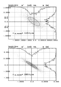
Figure 4: Horizontal phase space portrait of a bunch launched at 7.944 GeV with initial Gaussian rms  $\epsilon_x \approx \epsilon_y \approx 50 \pi \mu \text{m}$  and dE/E = 0. Top : end of the 21.2 GeV pass (collision energy), bottom : end of the the decelerated 7.9 GeV last pass.
