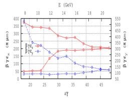
Figure 7: Evolution of the emittances in the presence of vertical orbit defect. Bunch recentered at linac only.
