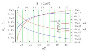
Figure 2: Energy dependence of cell tunes and chromaticities; the vertical bars materialize the 11 design energies.
