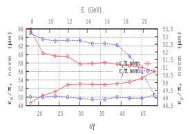
Figure 6: Emittances after each turn. The bunch is recentered at each of the six LSS.
