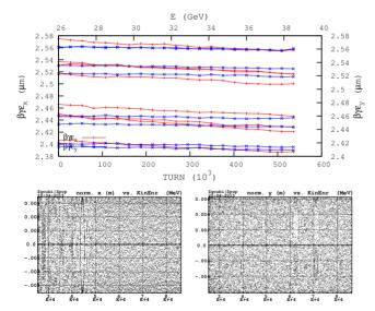
Figure 3: Observation at an IP. Top: normalized invariants over 500,000 turns. Bottom: turn-by-turn horizontal (left) and vertical (right) normalized excursions over 2 million turns.
