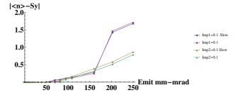
Figure 6: Polarization aperture with  $Q_y = 0.675$  and considering the addition of imperfection resonances of 0.1 at  $G\gamma = 62$  (Imp1) and  $G\gamma = 63$  (Imp2). We consider response for both nominal (pp run) and slower ramp rate by 2.22 (p-Au run).
