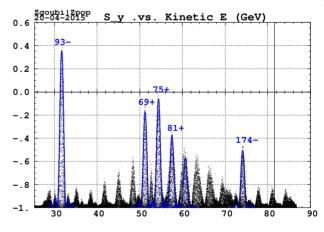
Figure 5: New optics. Turn-by-turn  $S_y$  values, 8 particles on 10 rms invariants are plotted. Envelopes (blue curves) are from theory.
