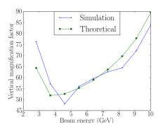
Figure 2: Misalignment magnification factor in the vertical plane for all passes from simulation compared with theoretical calculation.
