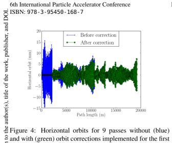
and with (green) orbit corrections implemented for the first pass.
