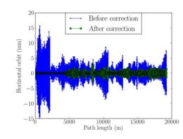
Any distribution of this work must maintain attribution to Figure 5: Horizontal orbits for 9 passes without (blue) and with (green) orbit corrections implemented for the first two 2015). passes.
