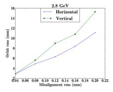
Figure 1: RMS of beam orbit distortion in eRHIC FFAG in both planes due to magnet misalignment errors, for the beam in the first pass with energy  $2.8 \ GeV$ .
