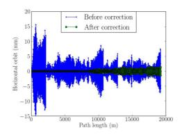
Figure 6: Horizontal orbits for 9 passes without (blue) and with (green) orbit corrections implemented for the first four passes.
