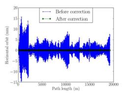
Figure 7: Horizontal orbits for 9 passes without (blue) and with (green) orbit corrections implemented for all the 9 passes.
