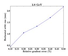
Figure 3: RMS of beam orbit distortion in eRHIC FFAG in horizontal plane due to magnet gradient errors, for the beam in the first pass with energy 2.8 GeV.
