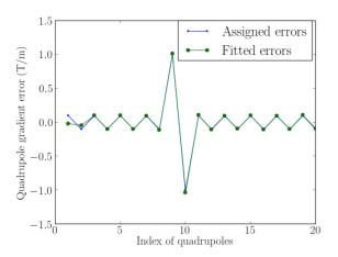
Figure 5: The comparison of the assigned and fitted gradient errors for 20 quadrupole magnets, for the case the orbit response matrix for all the passes were used in the simulation.
