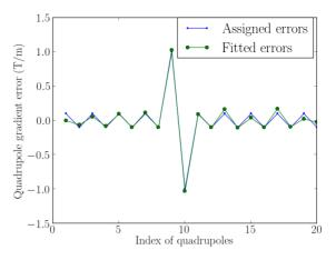
Figure 4: The comparison of the assigned and fitted gradient errors for 20 quadrupole magnets, for the case only the orbit response matrix for the first pass was used in the simulation.
