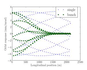
Figure 6: The comparison of the orbit response of the bunched beam and the orbit response of the on-momentum particle.
