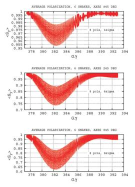
Figure 6: The simulation results for 6 snakes, snake axis as  $\pm 45$  degrees. From top to bottom, the vertical invariant is  $\epsilon_y = 1$ , 6,  $9\sigma$ , with  $\sigma = 2.5\pi$ mm.mrad normalized emittance. Each plot shows the average vertical projection of the spin, computed from the tracking of 8 particles evenly distributed on the invariant. The horizontal invariant is negligible. The polarization is preserved for all cases.
