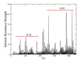
Figure 4: The intrinsic resonance strength of RHIC lattice for a particle on a  $10\pi$  normalized emittance invariant. Below 100 GeV, the resonance strength is less than 0.18. To accelerate proton beam to 250 GeV, the stronger resonance strength of 0.45 has to be overcome.
