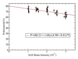
Figure 2: AGS polarization at extraction as function of bunch intensity. The polarized proton source can deliver intensity of  $9 \times 10^{11}$  at the Booster input. Booster scraping (both horizontal and vertical) is used to reduce the beam emittance for AGS injection. The intensity in this figure is changed by varying the Booster scraping level.
