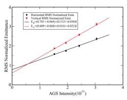
Figure 3: AGS emittance measured by IPM vs. intensity at the AGS extraction.
