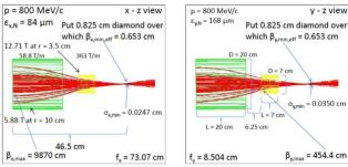
Figure 5: Quadrupole doublet half cell for final muon cooling with a flat beam,  $\beta_{x,y}^* = 0.55$  cm, and a 0.825 cm long diamond absorber. The G4beamline transmission is 995/1000 and the coverage for quadrupoles is at least  $\pm 3.0\sigma$ .
