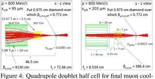
Figure 4: Quadrupole doublet half cell for final muon cooling with a flat beam,  $\beta_{x,y}^* = 0.65$  cm, and a 0.975 cm long diamond absorber. The G4beamline transmission is 998/1000 and the coverage for quadrupoles is at least ±3.1 $\sigma$ .
