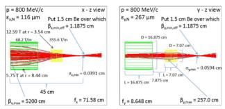
Figure 3: Quadrupole doublet half cell for final muon cooling with a flat beam,  $\beta_{x,y}^* = 1$  cm, and a 1.5 cm long berylium absorber. The G4beamline transmission is 996/1000 and the coverage for quadrupoles is at least  $\pm 3.0\sigma$ .
