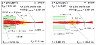
Figure 2: Quadrupole doublet half cell for final muon cooling with a flat beam,  $\beta_{x,y}^* = 1.25$  cm, and a 1.875 cm long berylium absorber. The G4beamline transmission is 998/1000 and the coverage for quadrupoles is at least  $\pm 3.2\sigma$ .
