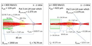
Figure 1: Quadrupole doublet half cell for final muon cooling with a flat beam,  $\beta_{x,y}^* = 2 \text{ cm}$ , and a 3 cm long LiH absorber. The G4beamline [10] transmission is 998/1000 and the coverage for quadrupoles is at least  $\pm 3.2\sigma$ . Coverage closer to  $\pm 4\sigma$  would be better.
