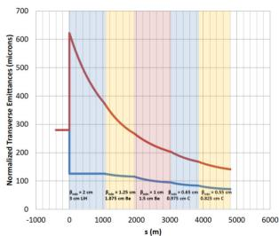
Figure 6: Transverse emittance versus channel length. The 6D xyz muon beam emittance is first transformed from (0.280, 0.280, 1.57) to (0.126, 0.622, 1.57) mm-rad and then cooled in five stages to (0.0714, 0.141, 2.418) mm-rad to meet the requirements of a muon collider. The total five stage channel length is 4808 meters and 62% of the 800 MeV/c ( $\gamma = 7.63$ ) muons decay. Less decay would be better.
