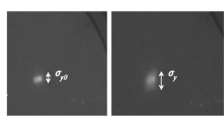
Figure 6: Beam spot as imaged with the MCP having the deflector turned off,  $\sigma_{v0} \approx 300 \,\mu m$  (left) and turned on,  $\sigma_{\rm v0} \approx 1000 \ \mu m \ (right).$
