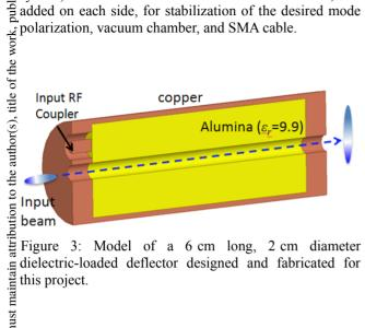
Figure 3: Model of a 6 cm long, 2 cm diameter dielectric-loaded deflector designed and fabricated for
