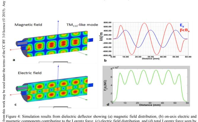
Figure 4: Simulation results from dielectric deflector showing (a) magnetic field distribution, (b) on-axis electric and magnetic components contributing to the Lorentz force, (c) electric field distribution, and (d) total Lorentz force seen by a 100 keV electron beam.
