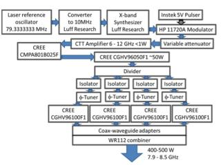
Figure 5: Simplified RF schematic for the solid-state Xband amplifier system developed for this project. DC supplies, computer control, diagnostics, and cooling systems are not shown.
