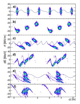
Figure 2: Phase space distribution at locations along the longitudinal merge: a) to e) are at the beginning of each stage and f) is at the end of the longitudinal merge. The rf fields at the corresponding places are shown in blue curves. Six representative bunches are shown.
