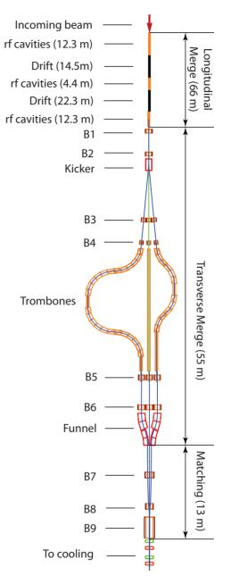
Figure 1: Merge Scheme. B1 - B9 are solenoid magnets for beam matching.
