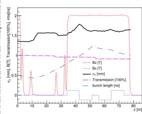
Figure 3: Evolution of  $\epsilon_T$ , rms bunch length and the transmission from end of the longitudinal merge to the end of the longest trombone.
