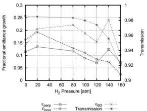
Figure 3: Emittance growth and transmission as a function of hydrogen gas pressure in the 12 m long transition channel. Emittance growth increases with reduced pressure; particle losses decrease with reduced pressure.
