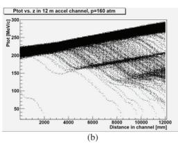
Figure 4: Particle momentum as a function of distance in the channel for  $H_2$  gas pressure of (a) 80 atm and (b) 160 atm. Particles falling out of the RF bucket are not properly accelerated and are excluded from the longitudinal emittance calculation.
