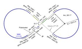
Figure 1: Top view layout of the ion ring.
