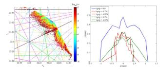
Figure 11: Tune footprint (left) and dynamic aperture (right) with distributed interleaved -I sextupole pairs.
