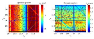
Figure 7: Horizontal (left) and vertical (right) DA at IP versus tune with non-interleaved -I sextupole pairs.
