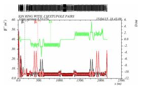
Figure 5: Modified ion ring optics with high beta at noninterleaved *x* and *y* correcting sextupole pairs.
