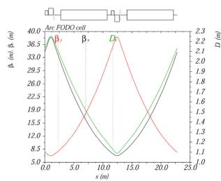
Figure 2: Ion arc FODO optics.
