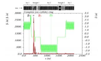
Figure 6: Complete ion collider ring optics.
