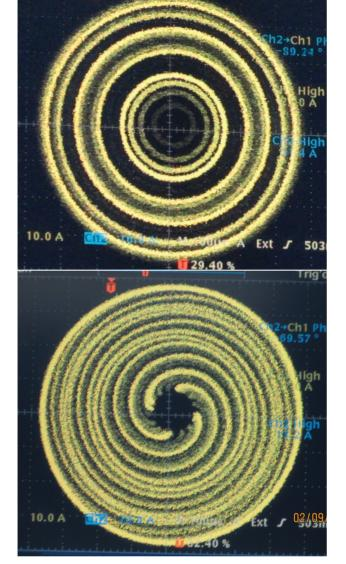
Figure 2: The raster amplitude waveforms observed by current viewing coils at the raster steering magnets for the concentric circle (top) and spiral (bottom) patterns with oscilloscope persistence for several macropulses.
