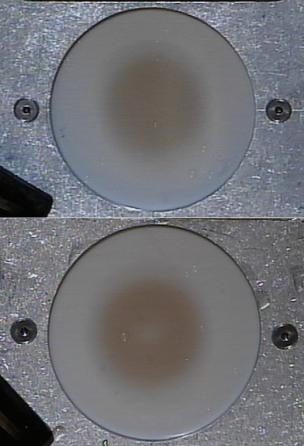
Figure 3: Beam spots at the IPF target produced using the concentric circle (top) and spiral (bottom) raster patterns measured by film irradiation.
