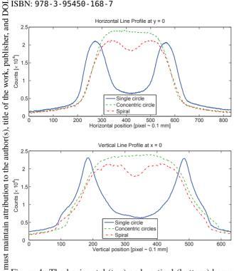
Figure 4: The horizontal (top) and vertical (bottom) beam work spot line profiles at the IPF target measured by foil irradiof this ation for single circle production (blue), concentric circle (green), and spiral (red) raster patterns.
