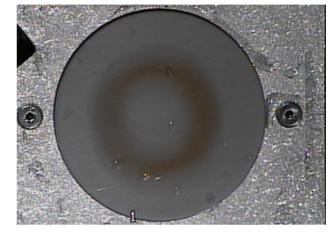
Figure 1: Beam spot at the IPF target with the single circle production raster pattern measured by film irradiation.
