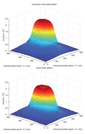
Figure 5: The beam spot at the IPF target measured by foil irradiation for the concentric circle (top) and spiral (bottom) raster patterns.
