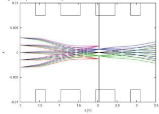
Figure 4: Angle cuts and matched rays in the *x* plane for a single-stage  $\times 10$  lens. Quadrupoles are indicated by the rectangles. Black curves: matched rays, no scattering; colored curves: scattered rays. The angle-cut collimator is represented by the vertical bars in the 3<sup>rd</sup> quadrupole.
