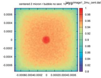
Figure 5: False-color simulated 12 GeV eRAD image of a 2 micron radius bubble in a 100 micron thick U slab, using a  $\times 50$  magnifier. Pixel size is approximately 0.2 microns (referred to the object). A "zoomed" 20  $\times$  20 flat-intensity rectangular beam was used to improve image statistics, which are better than with typical eRAD single bunches and a  $\sim 1$  millimeter FOV; the fall-off of image intensity at the border is an artifact.
