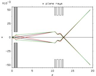
Figure 3: Matched and scattered rays in a  $\times$ 50 compound lens. Black: matched; red: positively scattered ray, green: negatively scattered ray.
