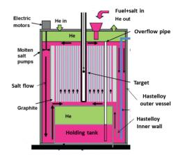
Figure 2: Cross-sectional view of GEM\*STAR reactor.
