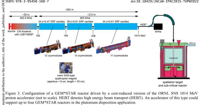
Figure 3: Configuration of a GEM\*STAR reactor driven by a cost-reduced version of the ORNL SNS 1014 MeV proton accelerator (not to scale). HEBT denotes high energy beam transport (HEBT). An accelerator of this type could support up to four GEM\*STAR reactors in the plutonium disposition application.
