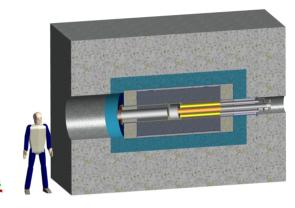
Figure 1: The IsoDAR target system and shielding. The target is a hollow centered cylinder surrounded by the FLiBe sleeve and a graphite reflector and cooled with water. The shielding in the current design consists of steel (shown in blue) and boron rich concrete (grey). A space for wobbler magnets is left in front of the target.
