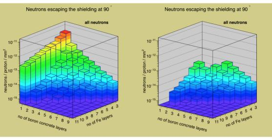
Figure 2: Neutron flux at 90 degrees for various material layers combinations (each layer is 10 cm thick). There are a number of possible material combinations for which the neutron flux is below  $10^{-13}$  n/p/mm<sup>2</sup> (right).
