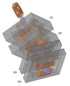
Figure 7: Preliminary assembly of the beam steering system installed on a 1 m long beam pipe.
