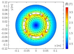
Figure 5: Quadrupole magnetic field distribution within the transverse cross-section plane.
