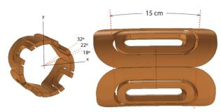
Figure 4: Three-dimensional layout of the SC quadrupole coils.
