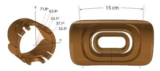
Figure 2: Three-dimensional layout of the SC dipole coils.
