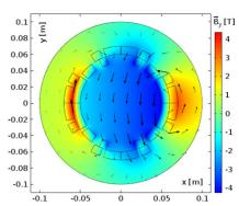
Figure 6: Bending magnetic field generated by the combined function magnet in the transverse cross-section.
