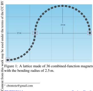
Figure 1: A lattice made of 36 combined-function magnets with the bending radius of 2.5 m.
