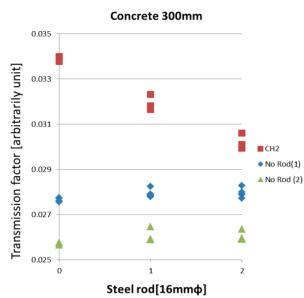
Figure 4: Transmission factor of iron rods in the concrete.
