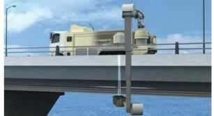
Figure 1: Transportable neutron source and 2D fast neutron detector.
