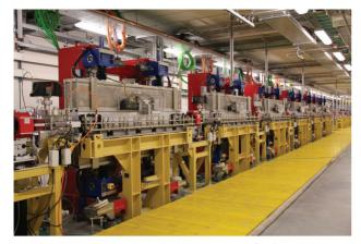
Figure 2: FEL1 EPU chain at FERMI@Elettra.
