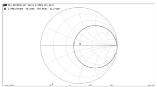
Figure 5: Smith Chart showing the overcoupling of the structure.
