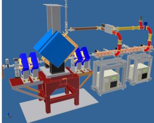
Figure 1: Layout of the TOP-IMPLART accelerator with the LEBT (left) and the first two SCDTL structures each one on his own table. The RF driving line is shown.
