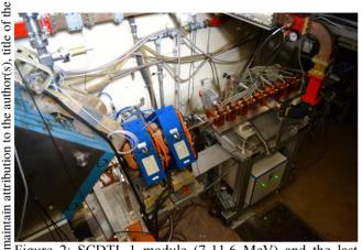
Figure 2: SCDTL-1 module (7-11.6 MeV) and the last must 1 part of the LEBT.
