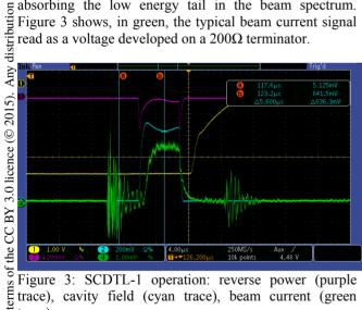
Figure 3: SCDTL-1 operation: reverse power (purple trace), cavity field (cvan trace), beam current (green trace).
