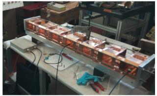
Figure 4: The SCDTL-2 structure on the RF bench under tuning. The structure is tuned before the last brazing, completing its construction.
