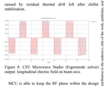
Figure 8: CST Microwave Studio (Eigenmode solver) output: longitudinal electric field on beam axis.
