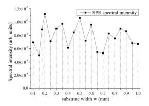
Figure 6: SPR spectral intensity as a function of the substrate width for the fixed corrugation depth a = 0.2mm.
