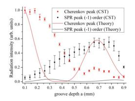
Figure 4: Radiation intensity dependence on a in geometry 1,  $r_1 = 0.3$  mm.
