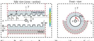
Figure 2: Geometry 2, a capillary with a radiation reflector.
