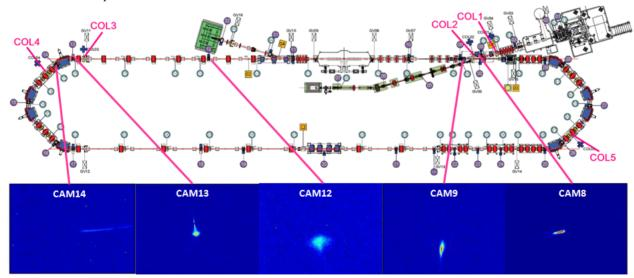
Figure 1: Layout of cERL. Collimators positions and tail profiles screen captures for laser phase +20 deg (42 ps tail).
