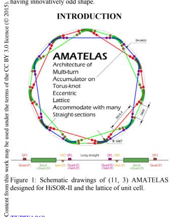
Figure 1: Schematic drawings of (11, 3) AMATELAS designed for HiSOR-II and the lattice of unit cell.
