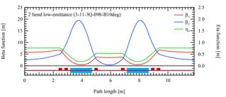
Figure 2: Optical function of (11, 3) AMATELAS for HiSOR-II storage ring.
