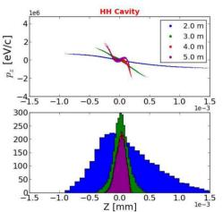
Figure 2: VB compression behaviour with the High Harmonic Cavity (HHC). The HHC is at 1.3 m from the cathode, the VB cavity at 1.5 m. Snapshots of the LPSs at 2, 3, 4 ant 5 m (top), and longitudinal binning - current distributions (bottom).
