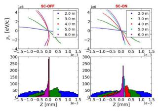
Figure 1: Snapshots of longitudinal phase spaces at 2,3,4,5, 6 m (VB starts a 1.5 m) during VB compression with SC ON and OFF (top), and macro particles longitudinal binning (bottom).
