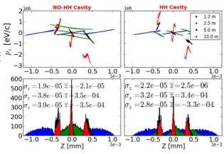
maintain attribution to the author(s). title of the Figure 3: Snapshots of longitudinal phase spaces at 1.2, 2.5, 5, 10 m from the cathode of a 3 bunch comb beam during VB compression with and without HHC (top), and macro particles longitudinal binning (bottom). work
