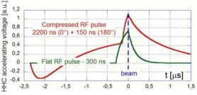
Figure 5: Harmonic cavity accelerating voltage profile.
