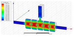
Figure 4: SPARC harmonic cavity model.
