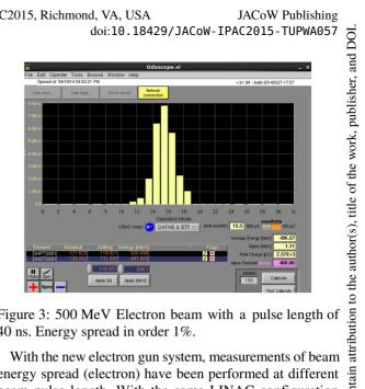
Figure 3: 500 MeV Electron beam with a pulse length of 40 ns. Energy spread in order 1%.
