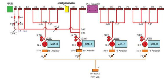
Figure 1: DAΦNE LINAC RF LAYOUT.
