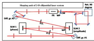
Figure 2: Setup of the 3-D pulse shaper; SLM – spatial light modulator, Diff. gr. – diffraction grating, WP – halfwave plate, CL – cylindrical lens, FR – Faraday rotator, CW – calcite wedge, Rot. 90 degree – laser beam rotator 90°.
