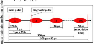
Figure 3: Time scheme of the scanning cross-correlator sused for 3-D laser pulse diagnostics. used for 3-D laser pulse diagnostics.
