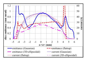
Figure 1: Beam dynamics simulation of electron bunches for photo cathode laser pulses with flat-top, Gaussian and 3-D ellipsoidal temporal profiles; normalized transverse slice emittance  $\varepsilon_{slice}$  distribution along the electron bunch.
