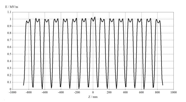
Figure 2: The field pattern of the  $\beta = 1$  RF-section. The strong cell coupling produces a very even field distribution that only drops a little in the end cells. The field peak in the centre is due to the input coupling there.
