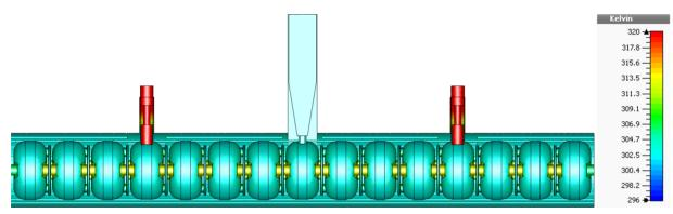
Figure 3: The thermal simulation of the  $\beta = 1$  structure as example. With the given design the iris temperature is  $\theta \approx 40^{\circ}$  C. The plungers can have a temperature of up to 80°C if they are fully moved inside the cavity without cooling. The temperature scale is cropped at 320 K to provide a better resolution of low temperatures.
